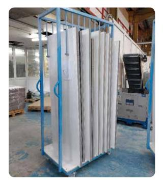
For example, Vista Panels invested further in the provision of bespoke racks and trolleys to ensure that large, bulky and heavy composite doors and other products can be stored and transported safely, significantly reducing manual handling risks.
